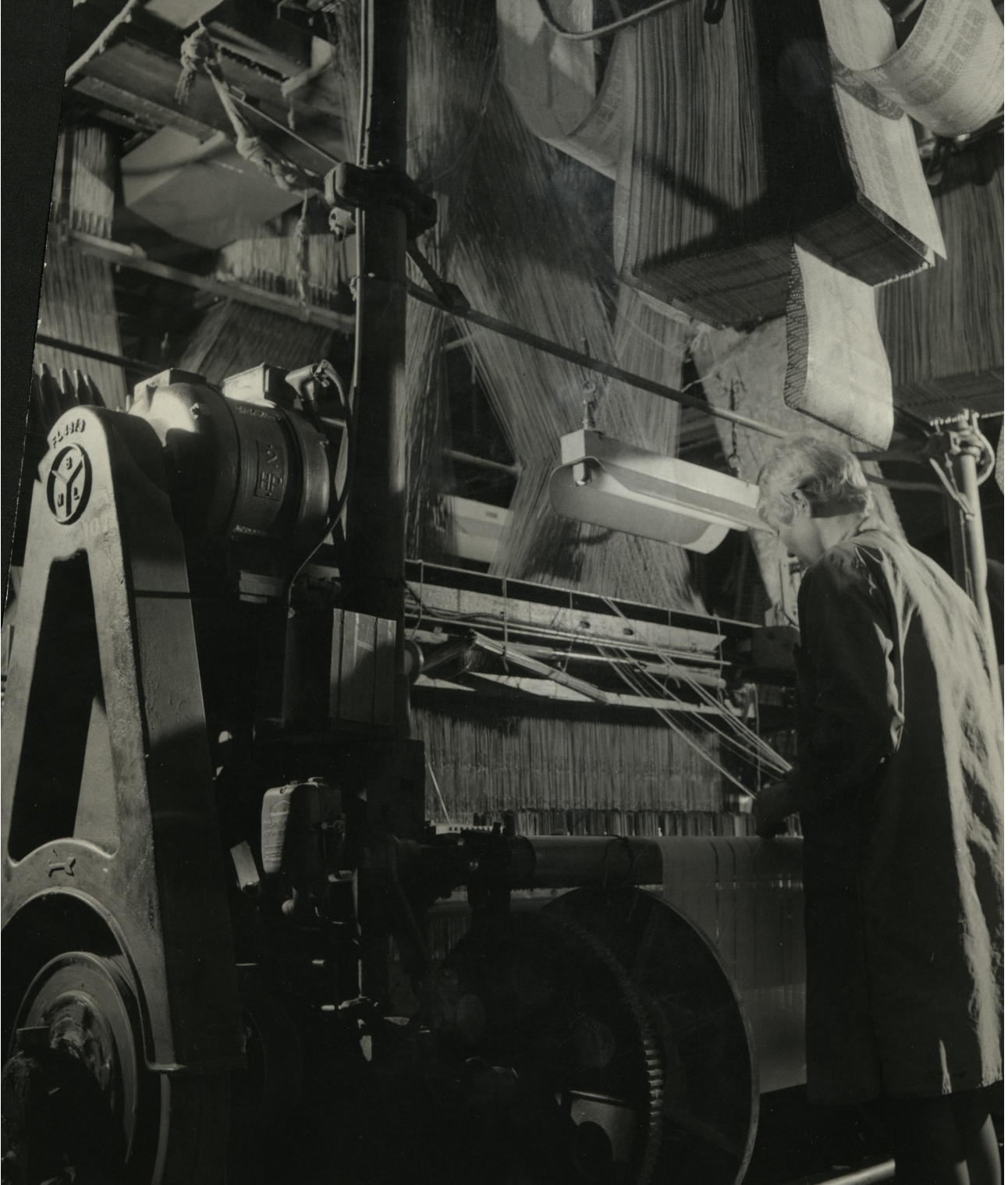
Jacquard loom in use for damask weaving, showing punched cards dictating the pattern of the cloth being woven, c.1960 (INF/7A/11/5/11)
